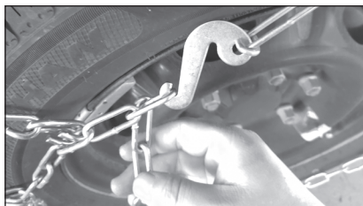
4. Hook the buckle on the outer side
