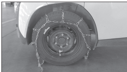
1. Hook an anti-skid chain to the tire
