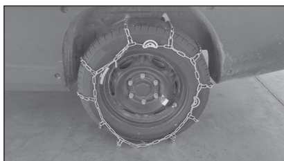
6. Tighten all the four buckles on the tire
