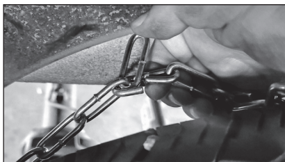
3. Buckle the inner side hook first
